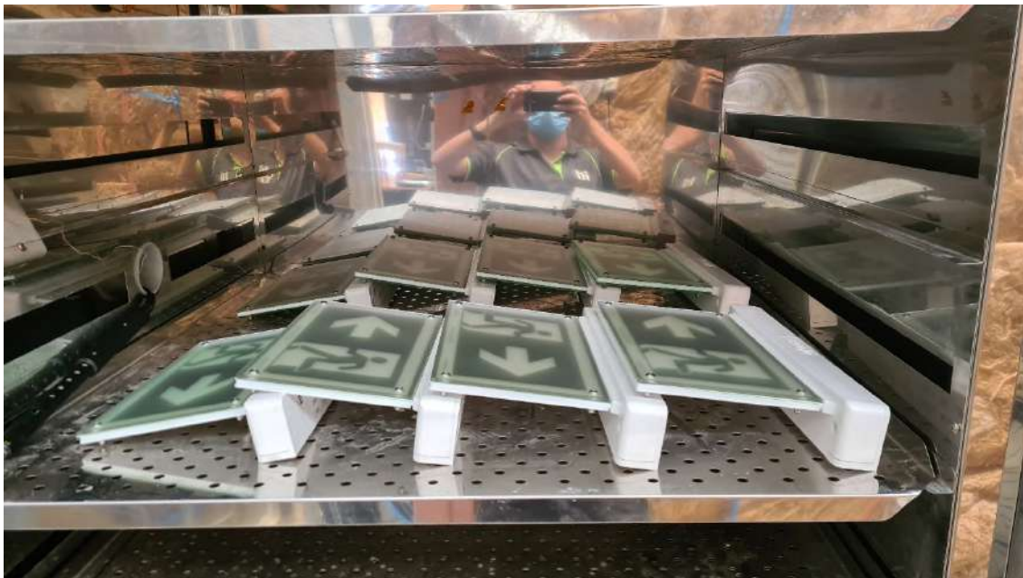
Figure 1: Samples in Environmental Chamber for Conditioning Test view.
