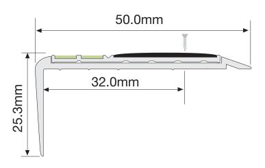
Ecoglo E22-075 Step Edge Contrast is adhesively fixed into the extrusion. The high visibility insert is manufactured from extruded 6063T6 aluminium section. Silicon Carbide anti-slip materials and custom made photoluminescent pigment are embedded in thermoset polyester carriers to integrally bond the active ingredients into the aluminium following curing at high temperature. The photoluminescent area is
