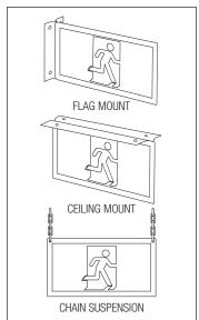
Ecoglo "Pictogram Left Arrow" S20 Signs are designed to clearly mark the direction of travel to the nearest exit. The signs will be clearly visible and readily understandable under all conditions of foreseeable use, including emergency conditions.
