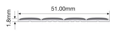
The N3-060 Anti-Slip/Step Edge Contrast is designed to both define the step edge and help prevent slips and falls in all weather conditions.
