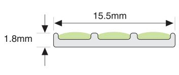
The G3-011 Anti-Slip/Step Edge Contrast is designed to ensure visibility of steps in escape routes for compliance with any performance based building codes. G3-011 will be effective in all light conditions including during failure of the main lighting.
