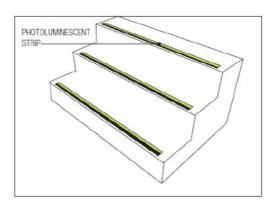
Step Edge Product Code: [E14-075] Description: [64mm wide aluminium (aluminum) base strip incorporating 10mm photoluminescent strip and 50mm black anti-slip strip. Available in lengths from 800mm to 1500mm in 100mm increments, or in full lengths of 2450mm or 3060mm.]
